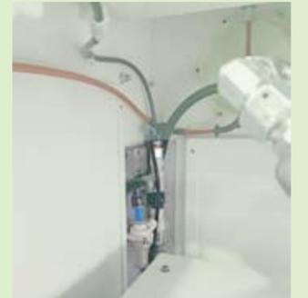
Vacuum generator installed inside the machine
