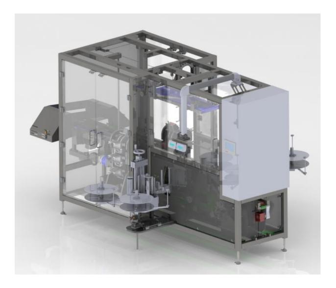
Bundling of individual packs into multipacks with side labelling provides customers with the flexible possibility of promotional packaging and provides consumers with an overview of the remaining packaging.
